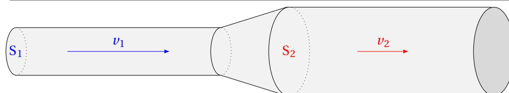
$$S_1 \times v_1 = S_2 \times v_2$$
